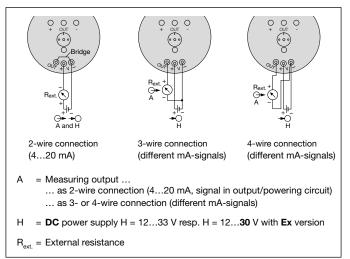
Fig. 7. Connection diagrams for 2-, 3- or 4-wire connection.
