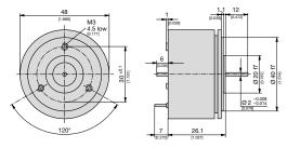
Fig. 2. KINAX 3W2 with special drive shaft at front and at rear. At front: Ø 2 mm [0.078"], length 12 mm [0.472"]. At rear: Ø 2 mm [0.078"], length 6 mm [0.236"].
