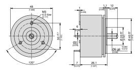
Fig. 4. KINAX 3W2 with special drive shaft at front and at rear. At front: Ø 6 mm [0.236"], length 12 mm [0.472"]. At rear: Ø 2 mm [0.078"], length 6 mm [0.236"].
