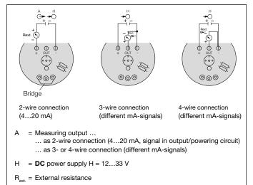
Fig. 11. Connection diagrams for 2-, 3- or 4-wire connection.
