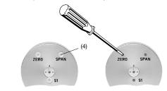
Fig. 12 Adjustments «ZERO», «SPAN» and «S1». Left: Adjustments covered by the sealing plug (4) Right: Adjustments exposed.
