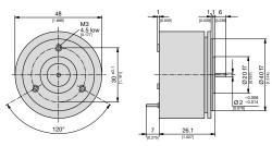
Fig. 1. KINAX 3W2 with standard drive shaft at front only, Ø 2 mm [0.078"], length 6 mm [0.236"].
