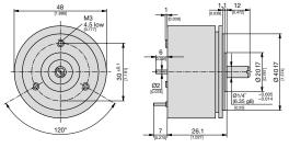
Fig. 6. KINAX 3W2 with special drive shaft at front and at rear. At front:  $\varnothing$  1/4", length 12 mm [0.472"]. At rear:  $\varnothing$  2 mm [0.078"], length 6 mm [0.236"].
