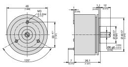
Fig. 3. KINAX 3W2 with special drive shaft at front only, Ø 6 mm [0.236"], length 12 mm [0.472"].
