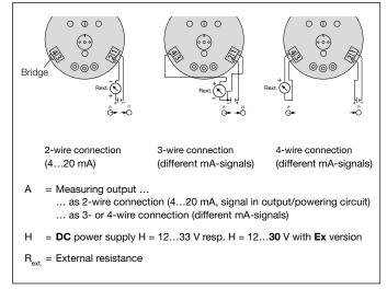
Fig. 9. Connection diagrams for 2-, 3- or 4-wire connection.
