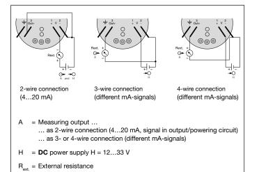
Fig. 10. Connection diagram for 4-wire connection.
